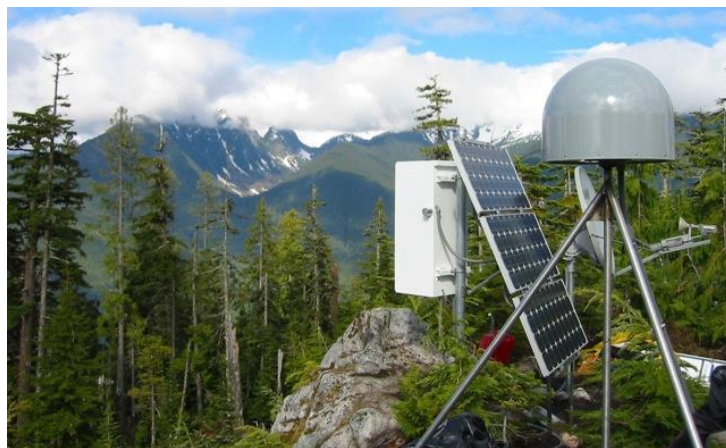
Figure 3. High-resolution GPS station (the dome), with solar charger and receiver. UNAVCO.
